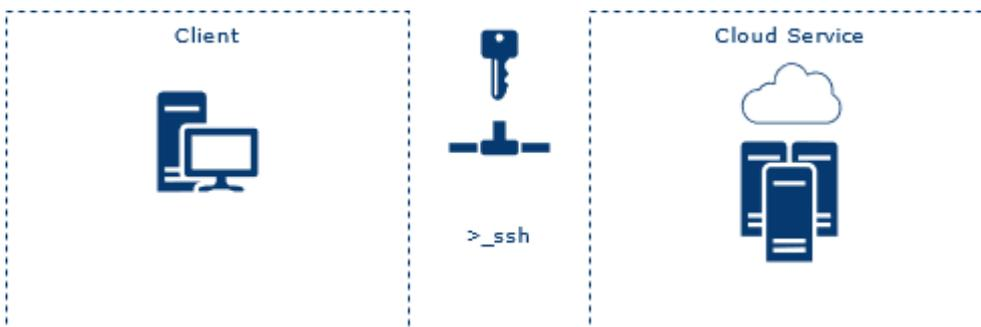
1. Client initiates the file transfer through SSH tunnel and tunnel is opened
