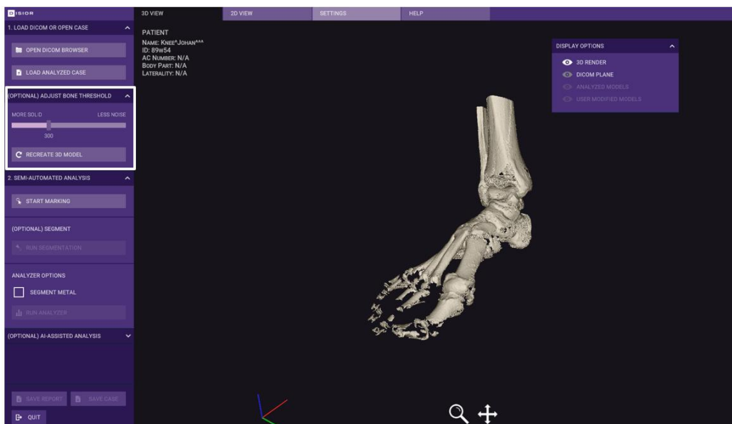
Image 3 You can change the threshold of the render by moving the 'BONE THRESHOLD' slider or typing a number and clicking 'RECREATE 3D MODEL'. Lower numbers include more data (more solid) and higher numbers include less data (less noise).
